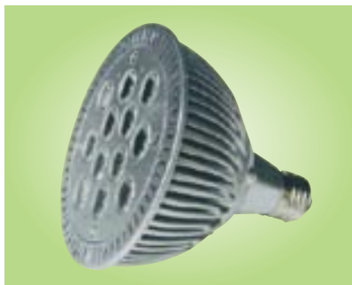
DLL1217 Base type: E27/B22 Light source: 12pcs 1w high power LED Input voltage: AC85-260V Power: 12W Size: 120*130mm Color: Cool/Warm white,blue,Green,Red, Yellow
