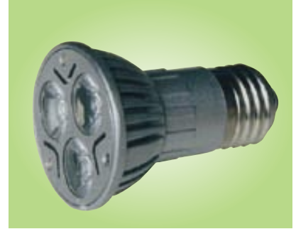
DLL1212 Base type: E27/B22 Light source: 3pcs 1w high power LED Input voltage: AC85- 260V Power: 3W Size: 50*75mm Color: Cool/Warm white,blue,Green,Red, Yellow
