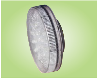
DLL1507 Base type: GX53 LED Q' ty: 36 Input voltage: AC110V/220V Power: 3.5W Size: 74*24mm Color: Cool/Warm white,blue,Green,Red, Yellow
